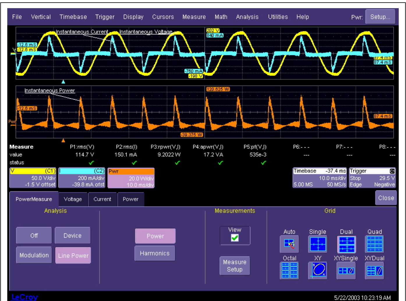
Figure 1 The elements of a power measurement (instantaneous voltage, current, and power) show on a WavePro 7300 using PMA2. Real and apparent power are automatically computed using parameters.
